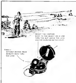
Figure 36. Method of determining azimuth of a visible object.
